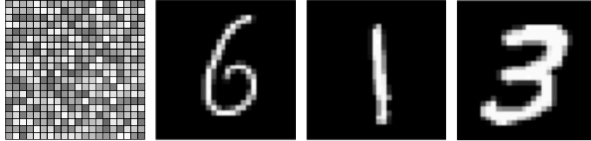
Figure 1. Images. An image is a function of two discrete indexes in which function values represent luminance. This information is arranged in a matrix \mathbf{X} in which the entry x(m, n) is the luminance at coordinates (m, n) [cf. (1)]. In this lab we work with images that represent handwritten digits [cf. (3)].
